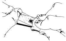
Lift the tucked-over end of tape and bridge it over the adhesive at approximately a 30-degree angle. With a piece of gauze, slowly make a single wiping stroke over the gage/tape assembly, bringing the gage back down over the alignment marks on the specimen. Use a firm pressure with your fingers when wiping over the gage, since the adhesive is quite viscous. A very thin layer of adhesive is desired for optimum bond performance.
